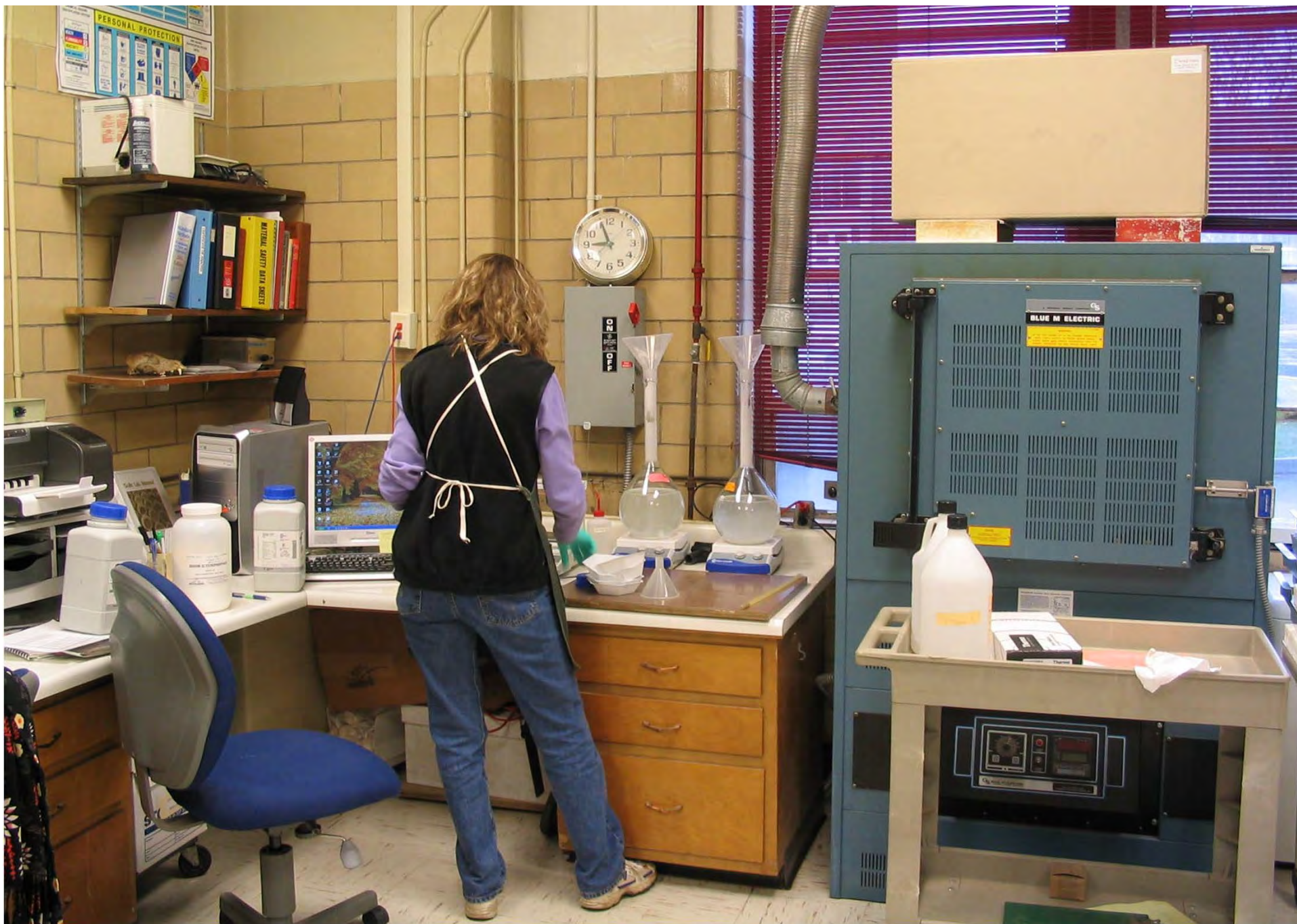
Making pH buffer solution used to estimate soil acidity for lime requirement determination.
