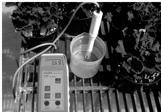
Figure 2. Portable electrical conductivity (EC) meters can be used to measure the EC of the dilute fertilizer solution to verify that the injector is working within the expected range. Compare the EC of the solution to that recommended on the fertilizer bag (Fig. 3) or the fertilizer label.
